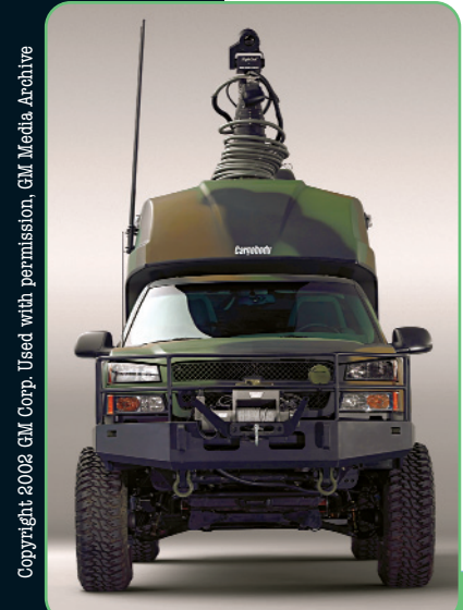
GM's hybrid military Silverado comes equipped with a fuel cell for silent auxiliary power.
